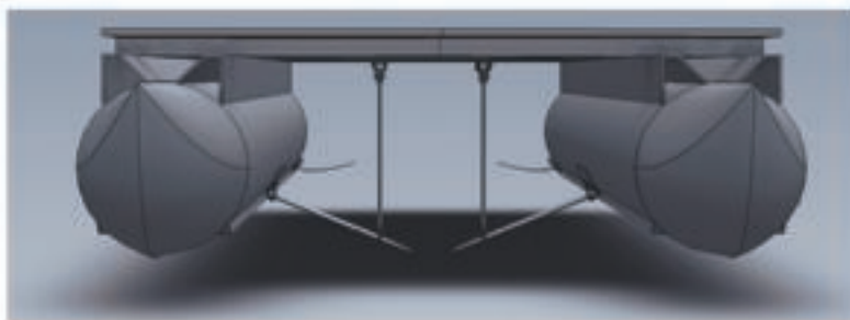
The Hydrofin's wings install just forward of the center of gravity via struts connecting to plates under the deck to resist upward water pressure.
